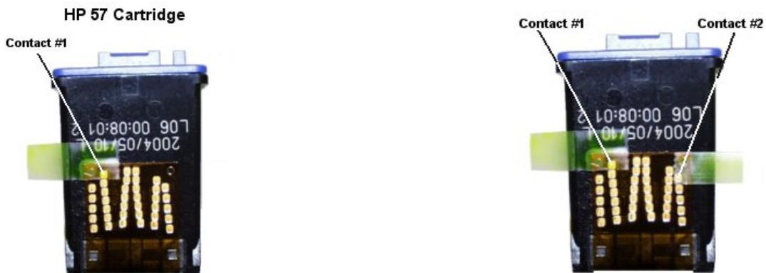
3. After the printer has completed printing off the alignment page, open the cover, remove the cartridge and place a piece of tape over Contact #2 as shown in the picture below.
