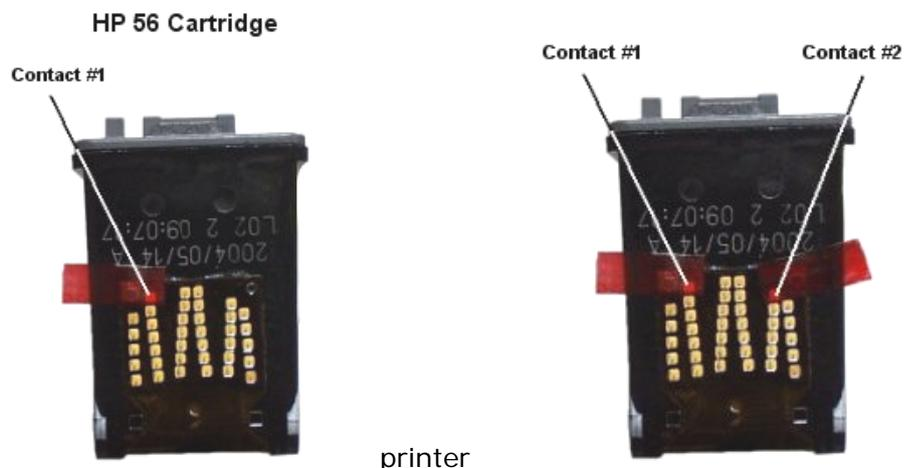
completed printing off the alignment page, open the cover, remove the cartridge and place a piece of tape over *Contact #2* as shown in the picture below.
